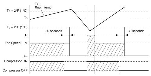
\* For 30 seconds after the compressor is turned OFF, the previous fan speed is maintained.
